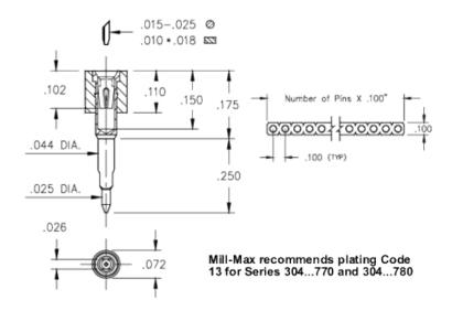
**Description:** Interconnect Socket Solderless Press-Fit Socket Accepts .015" - .025" (0,38 - 0,635 mm) dia leads Single Row Through Hole
